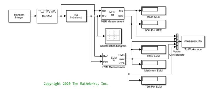
In this model, the I/Q Imbalance block sets the amplitude imbalance to 1 dB, the phase imbalance to 15 degrees, and the DC offset to 0. The MER Measurement block is configured to output the mean MER, and the 90th percentile MER. The EVM Measurement block is configured to output the RMS EVM (normalized to the average reference signal power), the maximum EVM, and the 75th percentile EVM.
