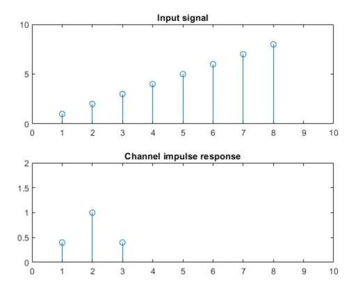
Compare the circular and linear convolution of u1 with h. Perform linear and circular convolution by using the conv and cconv functions, respectively. The smearing effects due to the nonideal channel cause the linear and circular convolution to yield different results at some points. A cyclic prefix (CP) enables effective use of OFDM in a nonideal channel with unknown propagation delay.
