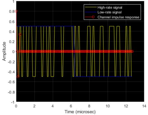
Low-Rate Signal, High-Rate Signal, and Channel Impulse Response
