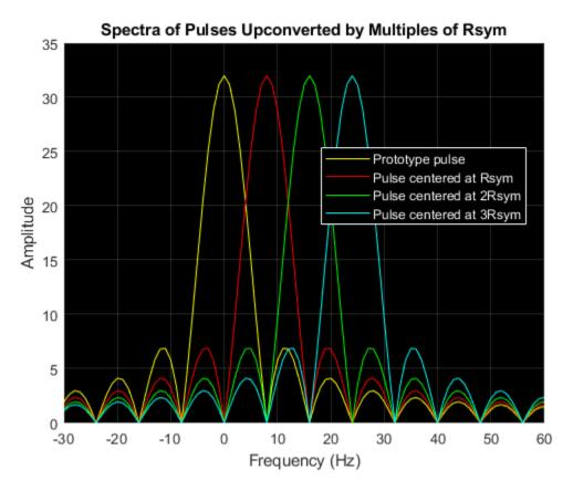
The frequency domain plot shows the orthogonal frequency translated pulses with spectral peaks of each subcarrier occurring at the zero crossings of all the other pulses.
